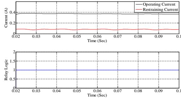
**Figure 13.** Operating and restraining currents in phase A and Relay logic for energization condition for low second harmonic contents
