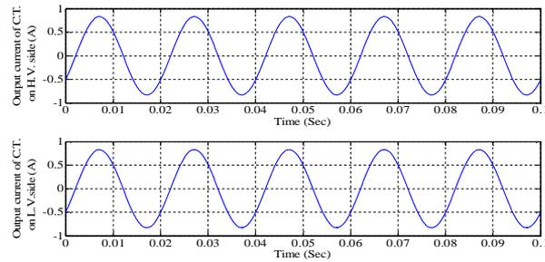
**Figure 3.** Instantaneous Values of currents on primary winding sides of CTs on H.V. and L.V. windings
