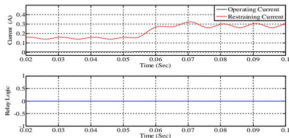
**Figure 9.** Operating and restraining currents in phase A and Relay logic for external fault condition
