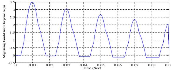
**Figure 10.** Waveform of Magnetizing Inrush current in phase A
