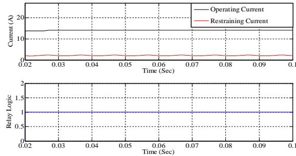
**Figure 8.** Operating and restraining currents in phase A and Relay logic for internal fault condition
