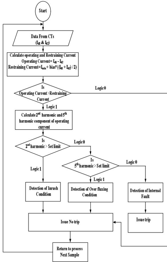
Figure 6. Flowchart of Implemented Differential Relay Scheme
