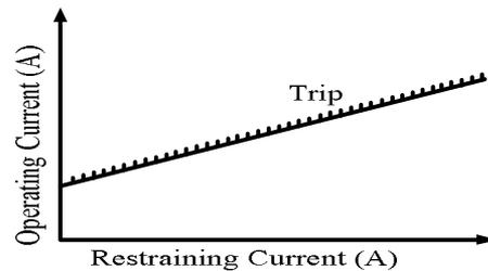
**Figure 5.** Biased differential relay characteristics
