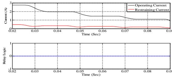
**Figure 11.** Operating and restraining currents in phase A and Relay logic for energization condition
