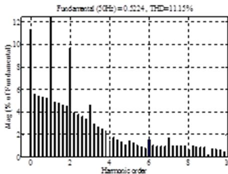
**Figure 12.** FFT Analysis of inrush current
