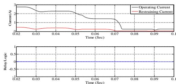
**Figure 14.** Operating and restraining currents in phase A and Relay logic
