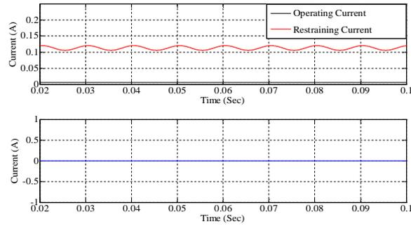
**Figure 7.** Operating and restraining currents in phase A and Relay logic for load condition
